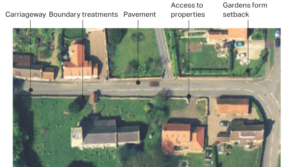
Secondary connector: A generally straight, well defined double lane approx. 5.5 metre wide single carriage with pavement on one side. Walls, narrow setbacks and fences create enclosure and space in the centre of Hemswell defining the street. Setbacks may vary from none to substantial. Strong edge is well maintained.
