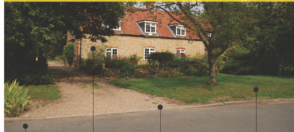
Carriageway Large garden Setback Kerb acts as a definition of public and private spaces Private space
