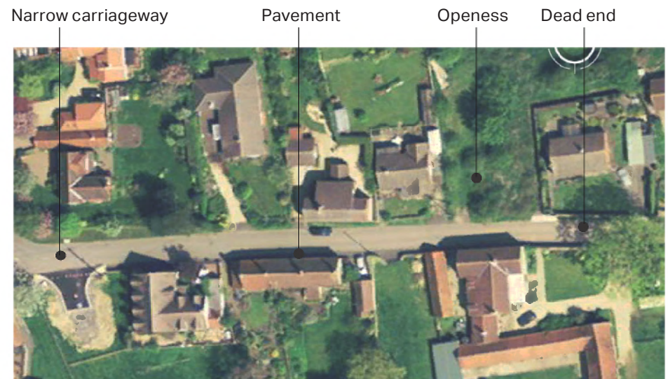
Mews, cul-de-sacs and access to dwellings arrangement: Have the narrowest carriageways only providing access to individual properties and having no through movement. This reduces vehicular movement and creates highly walkable streetscapes. There are a minimal amount of boundary treatments and the large setbacks create openness.
